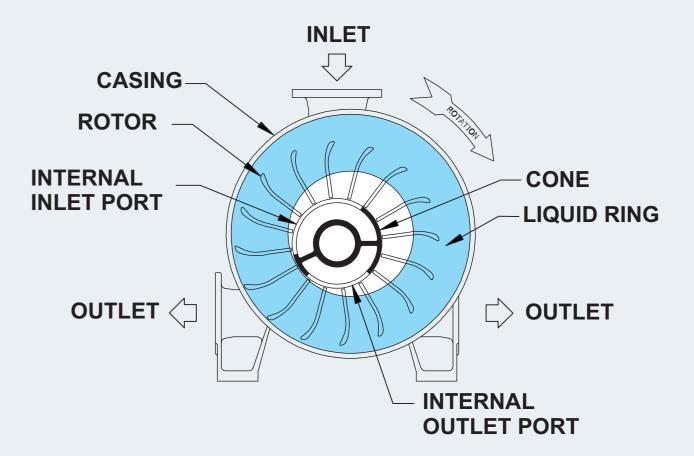
The pump's components are positioned in such a manner as to admit air when the rotor chamber is emptying the liquid, and then allowing the air to discharge once compression is completed. Sealing areas between the suction and discharge ports are provided, to close the rotor areas, and to separate the inlet and outlet flows.
