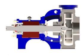
Disc pumps are used for difficult pumping applications such as liquids with abrasives, solids, high viscosity, entrained gas or air.
