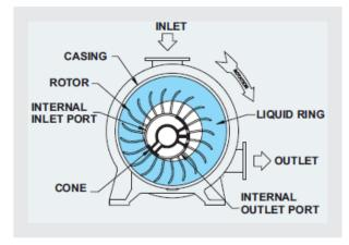
The pump's components are positioned in such a manner as to admit air when the rotor chamber is emptying the liquid, and then allowing the air to discharge once compression is completed. Sealing areas between the suction and discharge ports are provided, to close the rotor areas, and to separate the inlet and outlet flows
